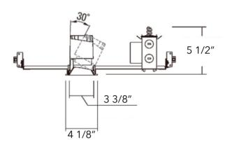
Ceiling Cut-out : Ø3-15/16"(Ø100mm) Mounting Frame : 12-1/16"(307mm) X 7-5/8(193.8mm)
