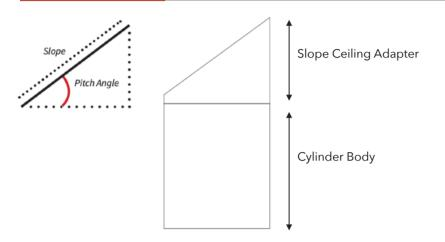
Slope ceiling adapter will be determined by the ceiling pitch angle. Adapter works with all cylinder sizes.
