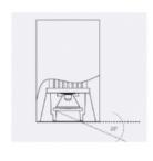
Low Output features a UGR <10.7 with 25 degree Shielding Angle
