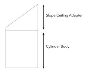
Slope ceiling adapter will be determined by the ceiling pitch angle
