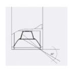
High Output features a UGR <17 with 45 degree Shielding Angle
